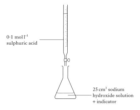
Volume of  $0.1 \text{ mol } 1^{-1} \text{ sulphuric acid required} = 22.5 \text{ cm}^3$
