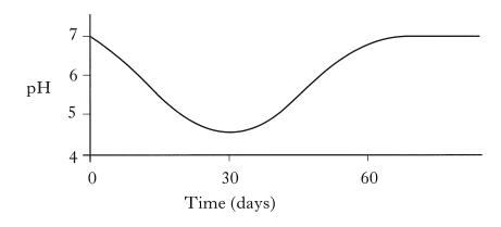
Describe and explain the pH changes taking place in the waste digestor over 60 days.
