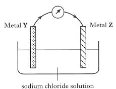
Which pair of metals would give an electron flow in this direction?
